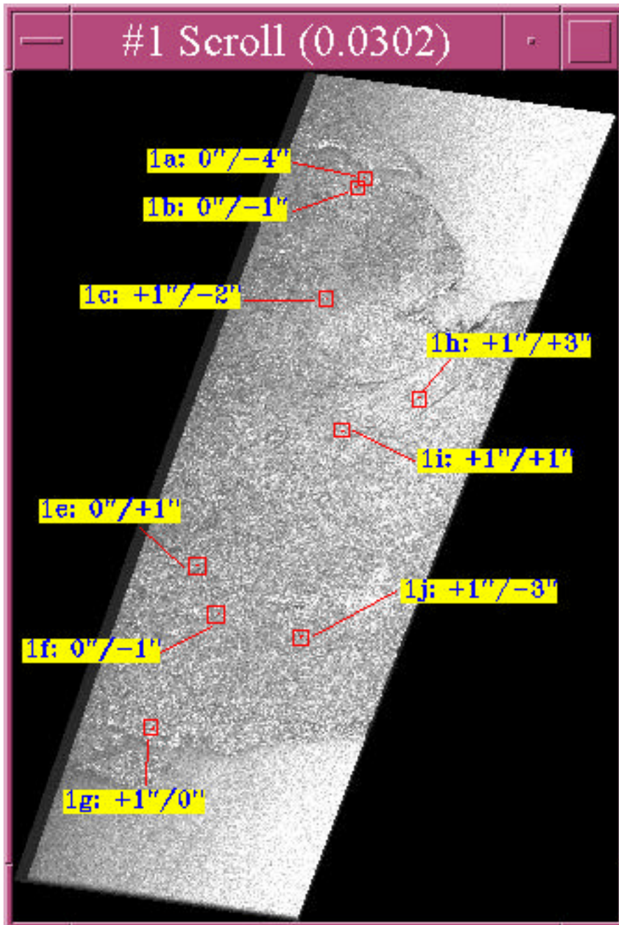
Figure 3. Points selected for validation on strip 1, together with their planimetric (x,y) deviation.
